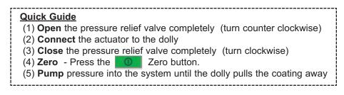
**1.** Ensure the pressure relief valve on the pump is **completely open**. (turn counter clockwise)
