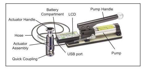
The *PosiTest AT* powers-up and displays dashes when the <u>0</u> button is pressed. To preserve battery life, the instrument powers down after 5 minutes of no activity.
