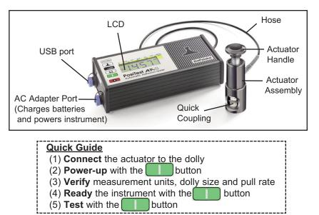
**1.** Place the actuator assembly over the dolly head and attach the quick coupling to the dolly by reaching through the holes in the actuator assembly and lifting the quick coupling. Release the quick coupling when the dolly head is completely engaged.
